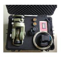
The angle at which its electronic fluxgate magnetometer reads a minimum value, is compared to a sighting through its optical theodolite. True north is determined by sighting a true north reference target mounted some distance away, or is derived from celestial navigation calculations on a sighting of the sun or another star.
