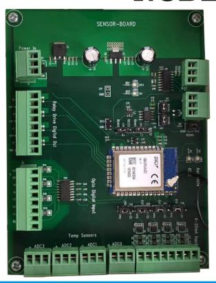
Nodelog is a low power analogue and digital I/O extension for Masterlog. It is designed to simplify cabling management in observation site.
